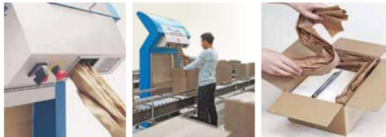
The converter forms single layer kraft paper into a high volume star-shaped paper configuration, which can be used as an effective filling material. It prevents products from shifting around in their box, ensuring damage-free arrival at the end destination. The converted paper gets dispensed directly at the point of operation, improving the efficiency of the packaging process and optimizing the speed of working.
